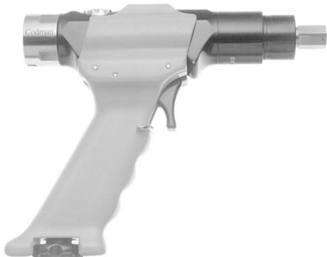
26-5000 CODMAN Modular Air Driver. Includes pistol grip handle, (26-5007) coaxial air hose and lubricant. Length 7" (178mm) Weight 20 oz. (567 gm) No load speed 20,000 rpm Braking time Within 1 sec. Power requirement 100 psi compressed dry nitrogen, nominal
