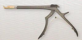
8 Test the reassembly to ensure smooth movement by squeezing and quickly releasing the handle and making sure the cutting edge of the crossbar comes flush with the footplate. If there is a gap, repeat the reassembly procedure. If the crossbar sticks or binds when the handle is squeezed, disassemble the instrument and check to see that it is clean and lubricated.
